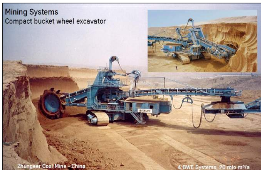
Bucket Wheel Excavator removing overburden in a Chinese coal mine. There's coal there somewhere. Really. Photo courtesy of ThyssenKrupp.
